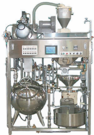
豆の浸漬→すりつぶし→煮沸 Dip → Grinding → Boiling
